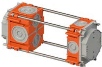
length of spacer bars = thickness of the wall to be built - 70 mm
