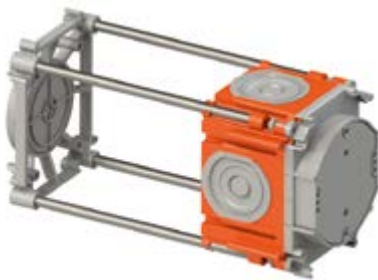
length of spacer bars = thickness of the wall to be built - 45 mm
